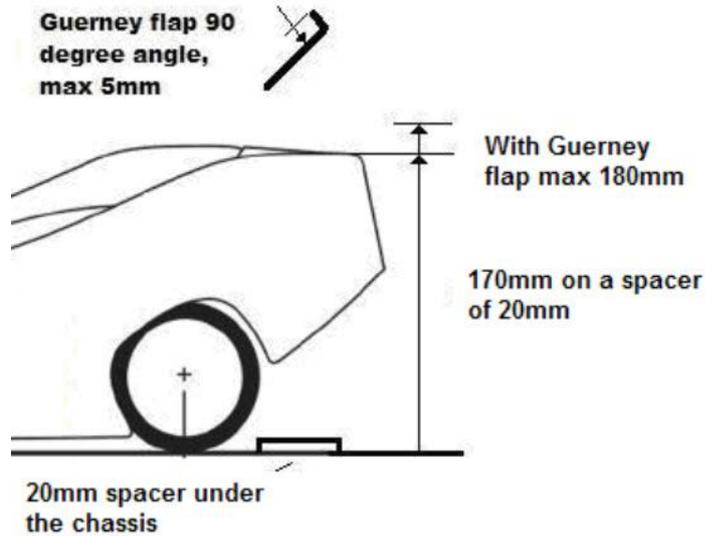
**Remarks:** The new rule concerning the offset of 100mm behind the rear axle and the farthest point of the body raises questions for the use of bodies with 2WD cars.
